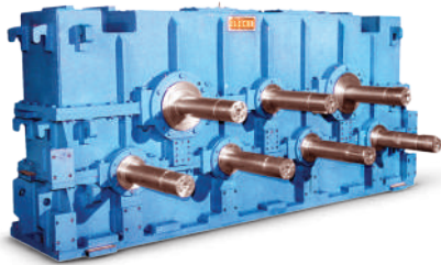
Hot Sizing Mill Gearbox with Two Input & Seven Output Shafts - Seamless Tube Plant
