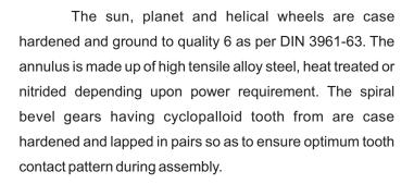
The casing is of welded construction mainly in two parts made out of Fe 410 WA IS 2062. The bearing bores are machined with high degree of accuracy on CNC machines.
