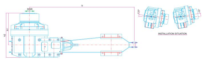
\* ACCORDING TO COUPLING AND MOTOR DIMENSIONS. SHAFT AND d1 WITH KEYWAY AS PER DIN 6885,PART-1,FROM-A. CENTRING DETAILS AS PER DIN 332, FROM-DS.
