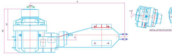
\* ACCORDING TO COUPLING AND MOTOR DIMENSIONS. SHAFT AND d1 WITH KEYWAY AS PER DIN 6885, PART-1, FROM-A. CENTRING DETAILS AS PER DIN 332, FROM-DS.
